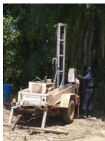
Figure 1: PAT 301TP drilling a 30 m borehole
