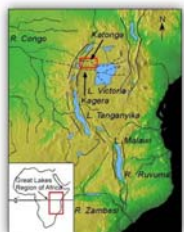
Figure 2: Digital elevation model of the Katonga region, prepared from SRTM data, showing the maximum historical elevation (1188 m asl) of static surface water based on Lake Victoria strandlines 3
